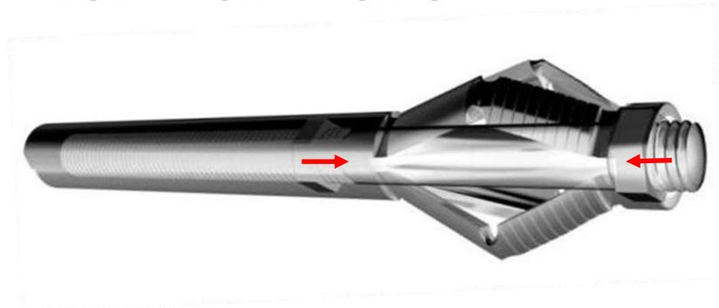
The X-BOLT® is an expanding bolt akin to a Chinese lantern with a central drive shaft. The opposing threads compress the expandable section from both ends to expand the wings perpendicularly to the shaft, without spinning, pushing or pulling the femoral head. Maximal expansion of the four wings is always easily seen on AP and lateral fluoroscopy.
